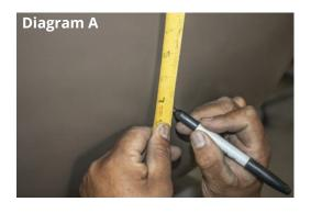
**Step 1.** Mark the spot where you want to make your hole. To find this spot, measure half way down the face of the bowl. Go down 1 inch. This will be where you will drill the hole.
