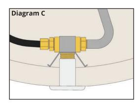
**Step 3.** Now that you have made your hole, you can begin to install the valve. From the outside, inset the chrome key valve cover. From the inside, you will place he securing bracket first, then the brass valve. You may stretch the securing bracket if needed (See Diagram C and D)
