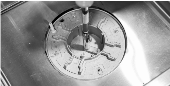
Loosen and remove the NG ORIFICE
